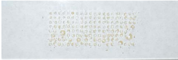
(c) Flux residue after removal of solder ball
