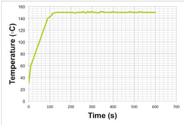
Figure 8. Curing profile of room temperature fast flow reworkable underfill
